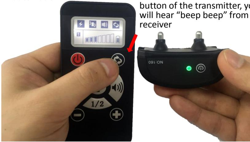
1.Press the “Automation” button of the transmitter, you will hear “beep beep” from the receiver
