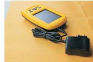
(1) The battery of this machine is the rechargeable lithium ion battery. If the machine is low battery, please charge for the battery. When cutting off the power supply fittings, you should grasp the plug and pull it out, not pull the power cord itself.
