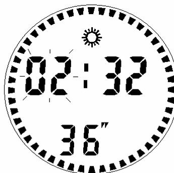
**2. Sea level pressure setting:** you can switch to this State by short pressing MODE button, In this state, long press MODE to choose to increase + (the default for the increase)
